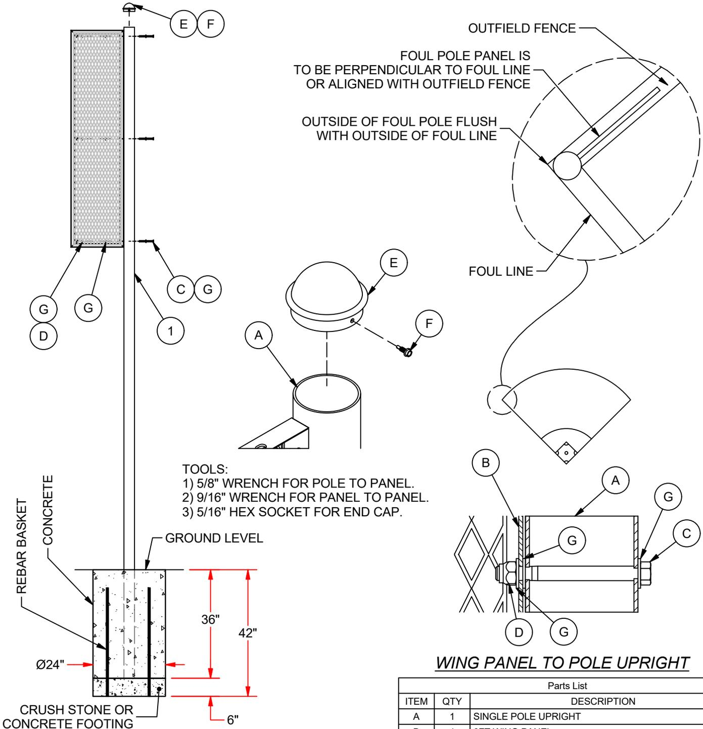
\* FOLLOW CONCRETE DETAIL AS SHOWN IF OPTIONAL GROUND SLEEVE IS NOT USED.
