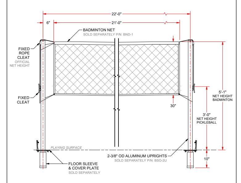
NOTE: UPRIGHTS CAN BE ANCHORED AND ALLOW FOR TENSIONING. INTENDED USE WITH 2.39" I.D. x 10" FLOOR SLEEVES INTO EXISTING 3.5" OR 3" SLEEVE BY USING THE APPROPRIATE SLEEVE INSERT ADAPTER, NOT INCLUDED.
