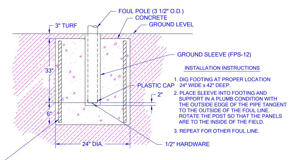
3/4" RE-BAR x 34", 6 PLACES PER FOOTING (NOT INCLUDED, TO BE PROVIDED BY INSTALLER). THESE ARE TYPICAL FOOTING DIMENSIONS FOR AVERAGE SOIL CONDITIONS.
