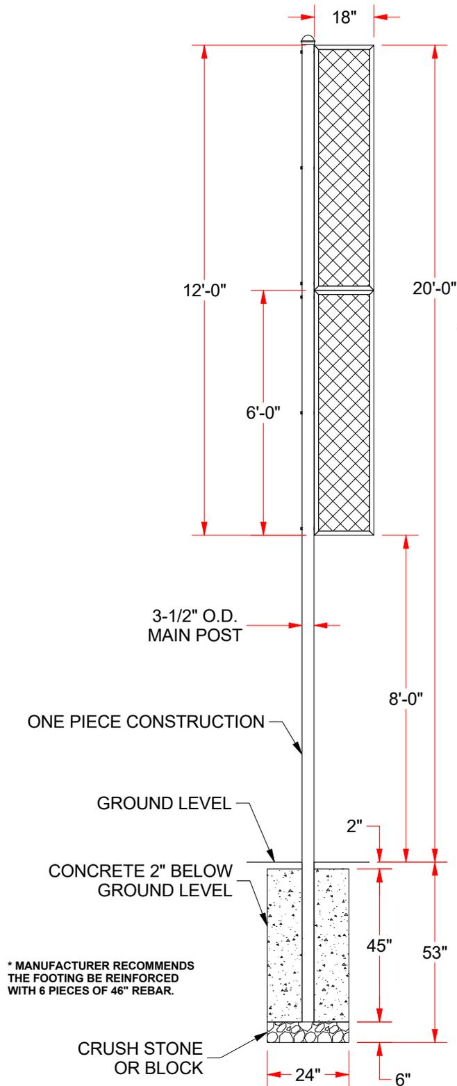
\* MANUFACTURER RECOMMENDS THE FOOTING BE REINFORCED WITH 6 PIECES OF 46" REBAR.
