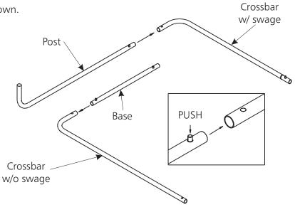
**4.** Weave assembled parts onto net as shown. Be sure to note the location of the top corner net tag.
